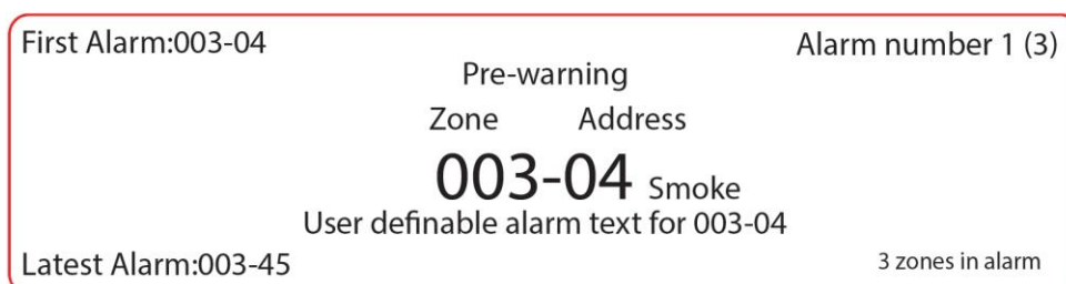
Figure 21: Pre-warning Alarm Display (pre-warning zone 003, address 04).
