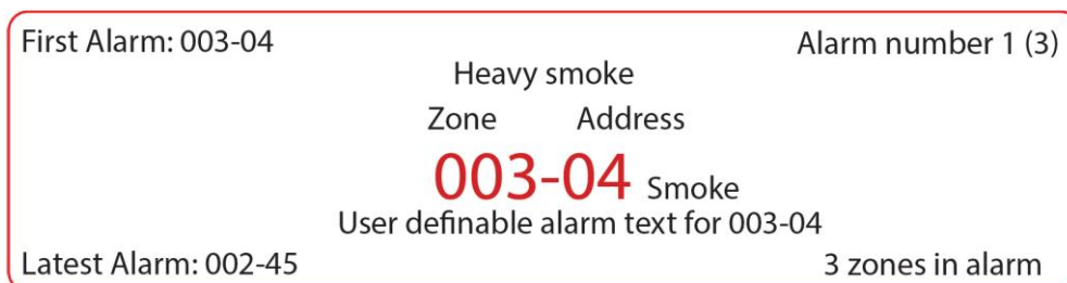
Figure 24: Heavy Smoke / Heat Alarm Display.
