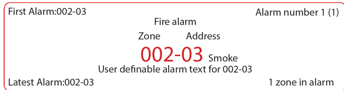
Figure 22: One Alarm Point Activating Fire Alarm (fire alarm zone 002, address 03).
