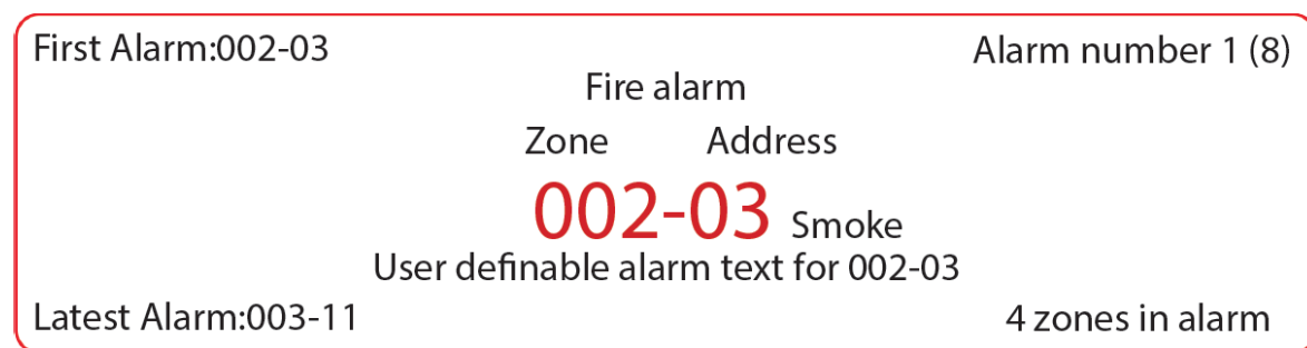
Figure 23: More than One Alarm Point Activating Fire Alarm.
